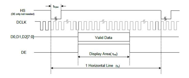
Horizontal input Timing at DE only mode
