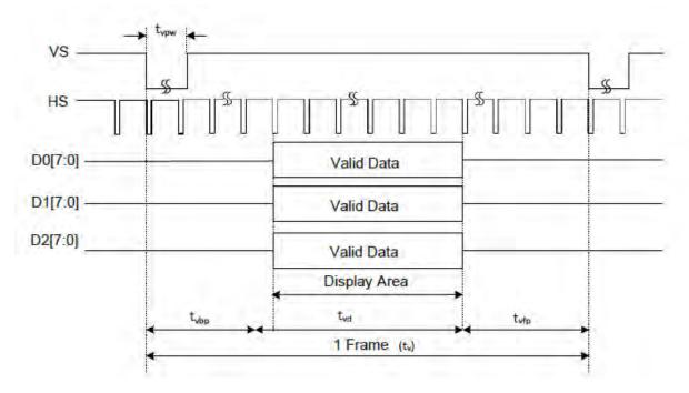
Vertical input Timing at Sync mode
